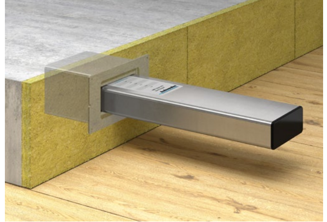
2. Remove shuttering, nails and transportation lock, apply max. 100 kg/m 3 mineral wool filler material. Insert the dowel.
