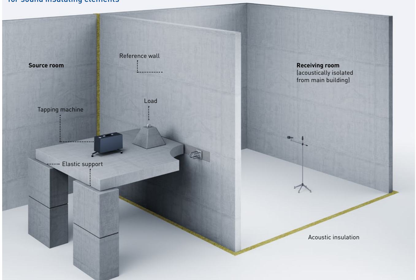
Schematic diagram of the measurement configuration at the Fraunhofer Institute IBP / EMPA for sound insulating elements
